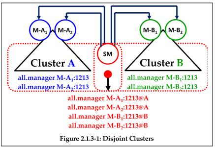
This mode of operation is correct as long as all of the managers are indeed replicas of each other. However, it is possible to construct a cluster whose members provide resources to two disjoint clusters, say A and B, as shown in the figure to the left. In this case, SM still
