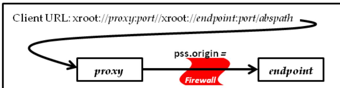
In the diagram the client prefixes the destination URL with the proxy location. The proxy server then contacts the specified endpoint on behalf of the client. The client is free to specify any valid endpoint. This mode is most suitable for outgoing connections and poses certain [security issues](#) that are described in a subsequent section. A valid destination URL must specify the `xroot` or `root` protocol element.
