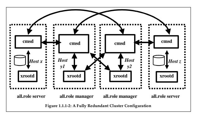
In order to provide a fully redundant service, all servers may be replicated and cross-connected, as full full crossbar configuration shows above.
