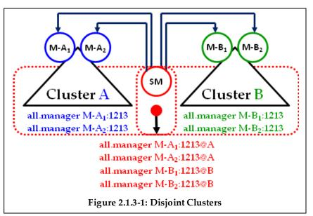
This mode of operation is correct as long as all of the managers are indeed replicas of each other. However, it is possible to construct a cluster whose members provide resources to two disjoint clusters, say A and B, as shown in the figure to the left. In this case, SM still
