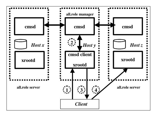
In the diagram, there are three hosts: x, y, and z. Host y serves as the redirector. Hosts x and z are the hosts that can be used to serve data to clients. Consequently, host y runs a manager **cmsd** while hosts x and z run server **cmsd**'s.
