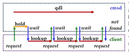
The left–side graphic illustrates the relationship between the **hold** and **lookup** delay and the **qdl** (i.e. query deadline) value. Initially, a client makes a file-oriented request (e.g. open, stat,
