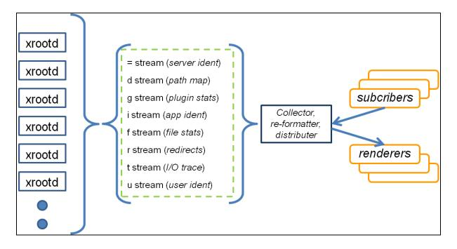
Because **XRootD** monitoring data uses a common compact format it is easy to collect and cross-reference. A collector would reconstruct the streams to contain relevant data for each type of subscriber in the desired format (e.g. JSON). A collector could also push preset data streams to known renderers like dash boards.
